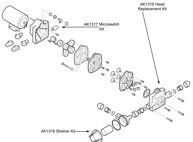
Note: UF models replaced UP codes. UF models come with Quick Connect 15mm heads. This head can be retrofitted to UP models using service kit AK1316
