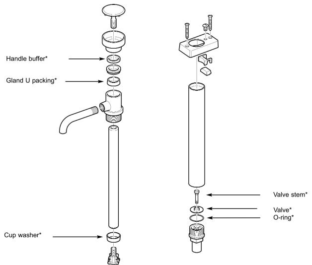
Pump replaced in 1993 by V Pump Mk 6 (see page 4)
