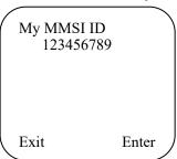
When you input 9 digits, Turn the coding knob to choose the number from 1-9, you need to input all numbers from the left to right one by one When you input all 9 digits then press the enter to confirm.
