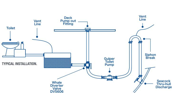
NOTE: WHERE DISCHARGE IS BELOW THE WATER LINE, A SIPHON BREAK MUST BE FITTED.
