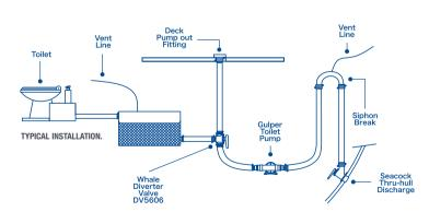
NOTE: WHERE DISCHARGE IS BELOW THE WATER LINE, A SIPHON BREAK MUST BE FITTED.
