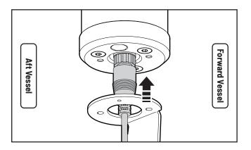
**Step 4**Mount lamp to bracket. The install is finished
