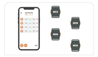
**11.** Ensure all OLAS transmitters are switched on and transmitting by checking the ID numbers on the home screen.
