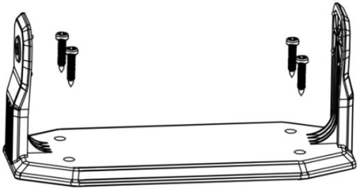
1. Place and fasten the mounting bracket on the console by 4 screws;
