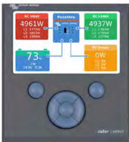
Color Control Panel, showing a PV application
