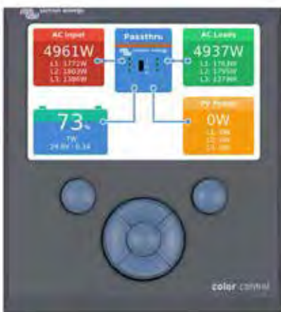
Color Control panel, showing a PV application
