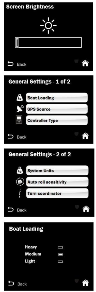
5. You may adjust the screen brightness according to your preference, by using the left and right directional buttons to set the brightness at a low or high level accordingly.
