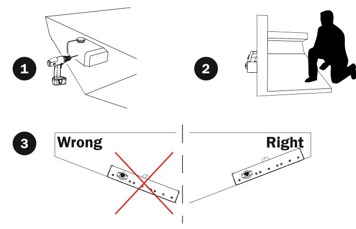
A good hint is that the closer the units are to the water line, the best the bank control of the boat will be (Figure 3).
