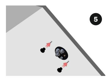
5. Mount the 4DHC Controller from the internal of the cockpit, with the given plastic screws
