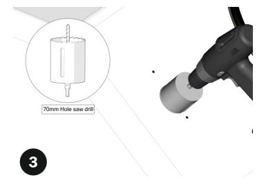
3. Create the central hole with a Ø70 saw drill
