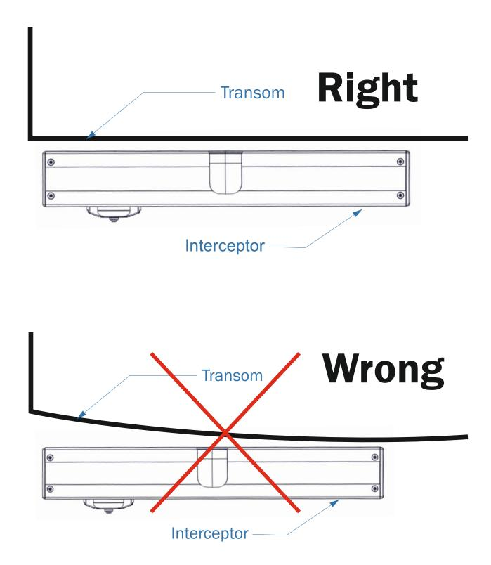
If the boat's transom has a significant curvature, it is necessary to create a flat plane for the installation (acceptable flatness tolerance: 2mm).
