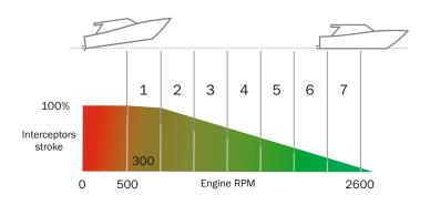
At each of the 7 steps wait for the speed to stabilize and then adjust the interceptors level until the maximum speed is achieved.
