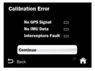
26. If at any step of the calibration procedure, an error occurs, the process will not be completed until the issue is resolved.
