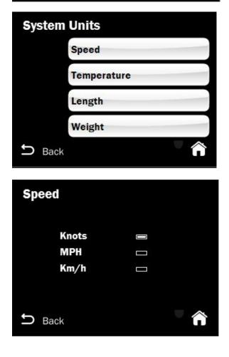
11. The System Units screen allows you to select the units that will appear in the 4DHC menu screens, for the Speed, the Temperature, The Boat Length and Weight
