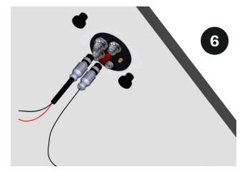
6. Mount the connection plugs in the 5-pole ports
