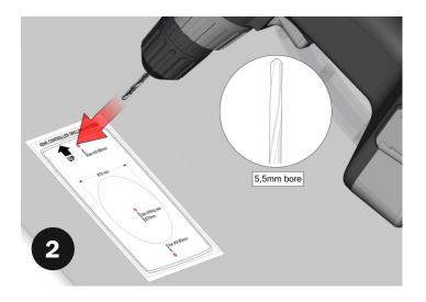
2. Drill the 3 holes according to the provided drilling pattern with a 5,5mm bore
