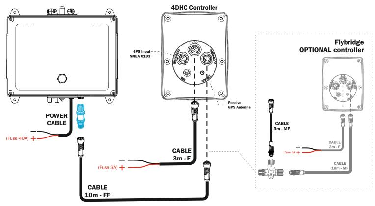
In case a new NMEA 2000 instrument to be added, a proper NMEA Network must be built.
