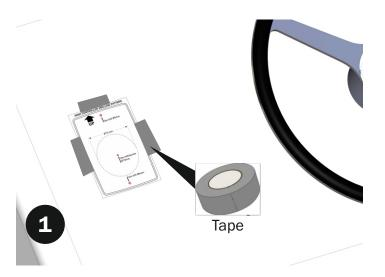
1. Place the 4DHC Drilling Pattern in the desired position (preferably a clean and easy-to-access area near the steering wheel of the boat, and with max. inclination angle at 80°).
