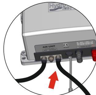
Cut the 8mm pipe at the proper length and connect it to the Air Unit
