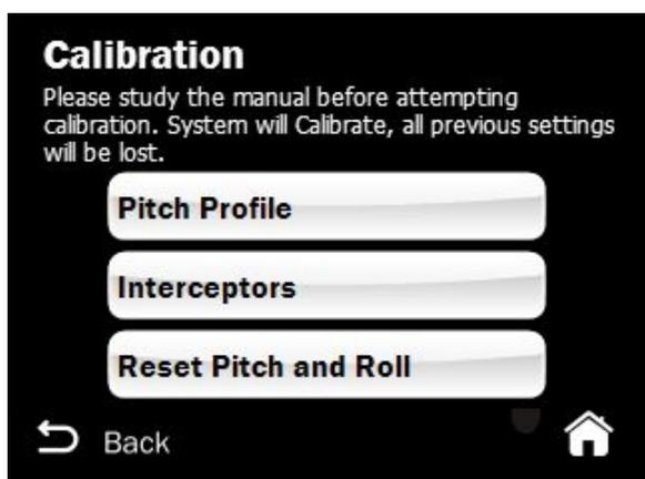
19. The Pitch Profile procedure adjusts the position of the interceptors for variable speeds, and it determines the pitch level of your boat during **Auto-Pitch** and **Full Auto** operating mode.
