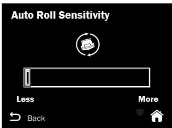
16. This option provides the ability to adjust the system automatic roll sensitivity according to your needs. Higher sensitivity, increases the response of the interceptors.
