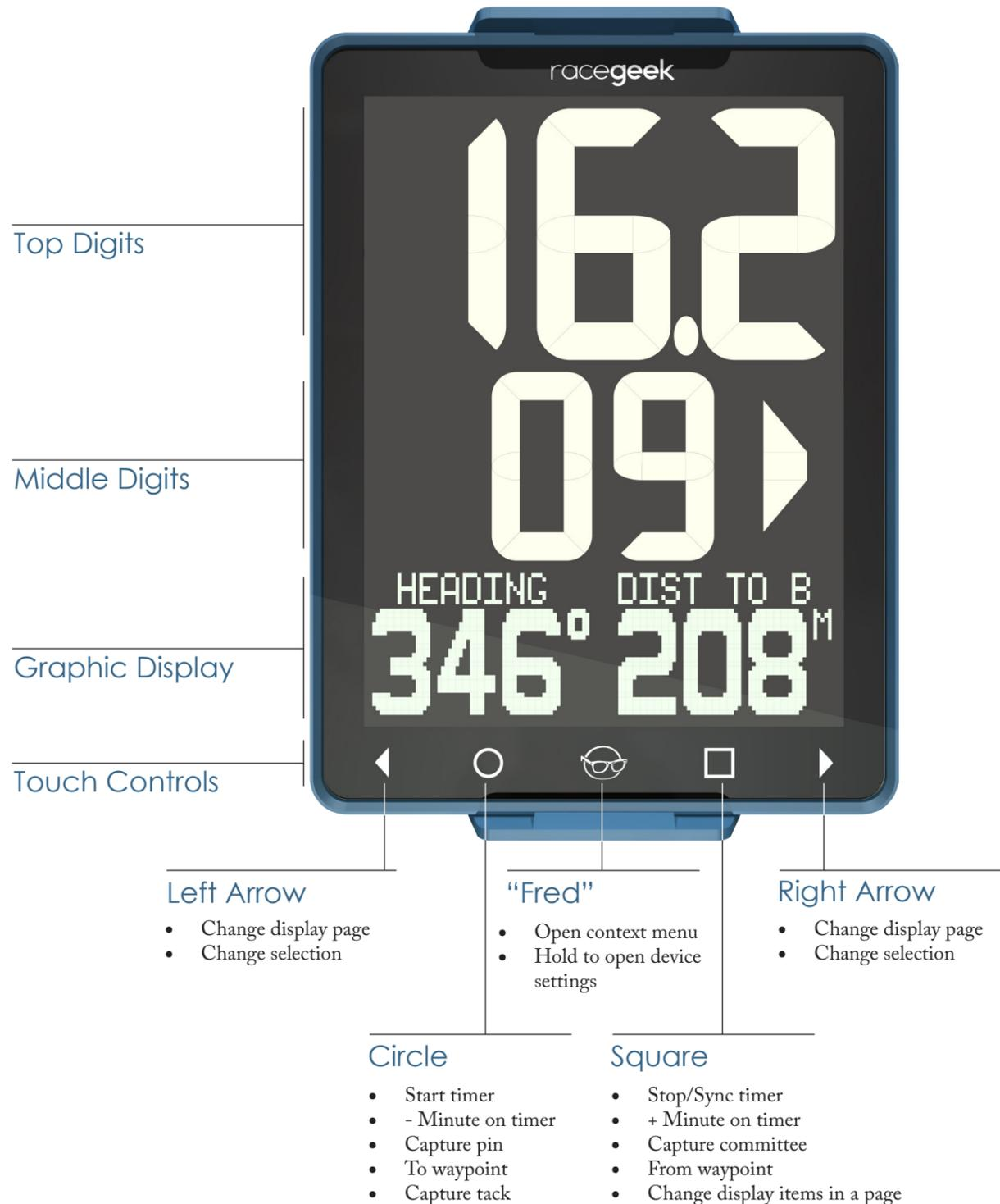
To change pages touch the left arrow (◀) or right arrow (▶) in the touch controls. You can cycle through the screens back to your original screen by continuing to touch the arrow in either direction.
