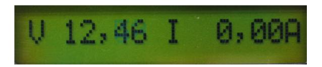
In the display mode you can see above the battery voltage and the charge current. The total current (wind and solar) is shown.
